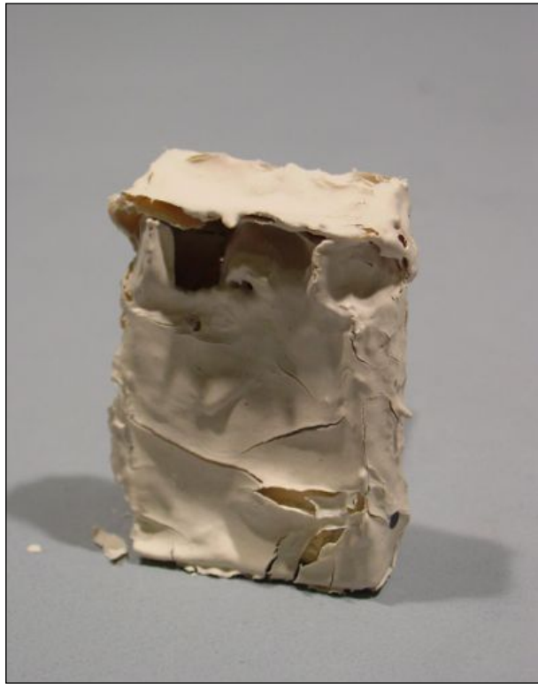
Pack with addition of paper fiber Note: Stronger final product than nylon fiber however not as strong as Wollastonite.
