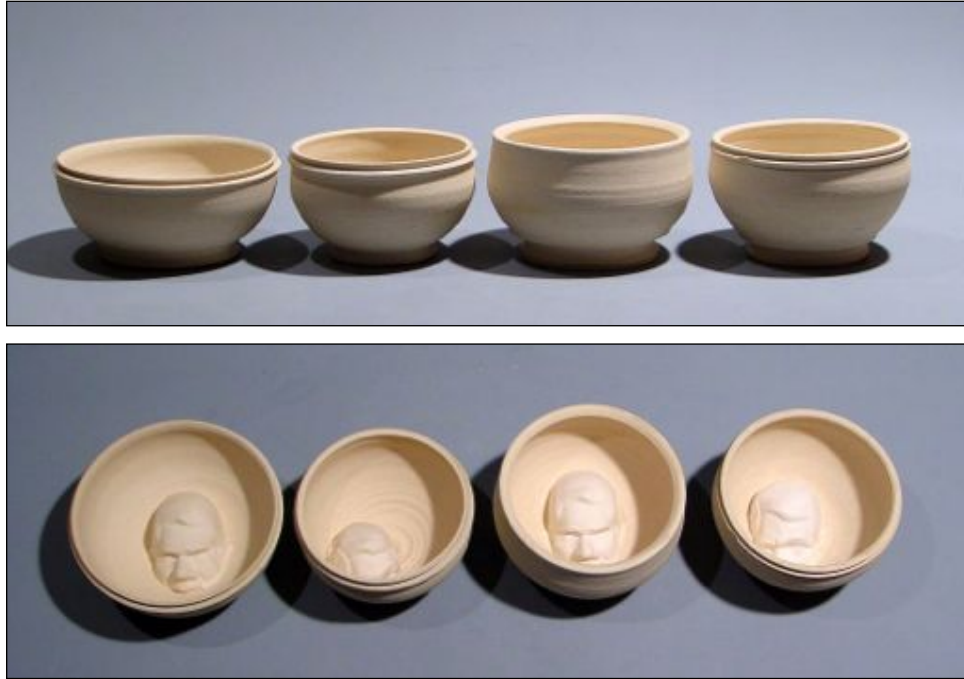
Series of tests. All bowls were thrown using #570 boxed clay. Castings inside the bowls from left to right: Original #570, #570 Revision 1, #570 Revision 2, #570 Revision 3.
