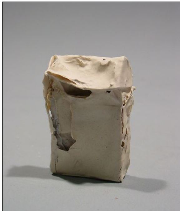
Pack with addition of Wollastonite. This was the strongest of tests, with the least cracking on surface. However, the Wollastonite also disrupted the texture of the slip.
