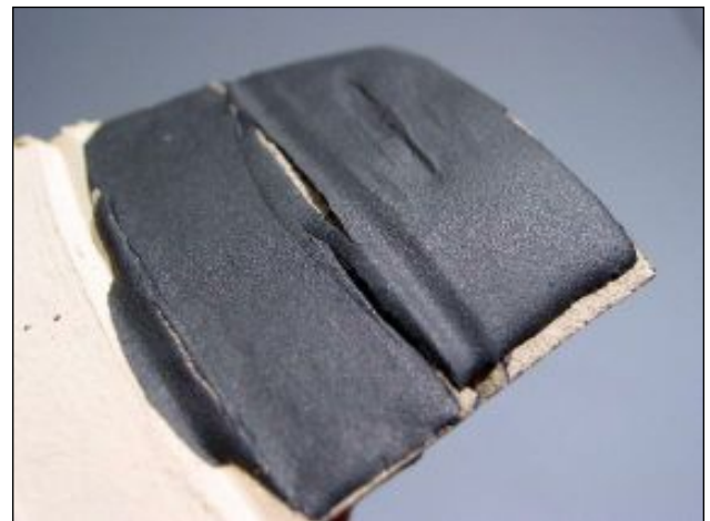
Detail of Mason Best Black in New Zealand base shows the curling and separation of slip from clay body
