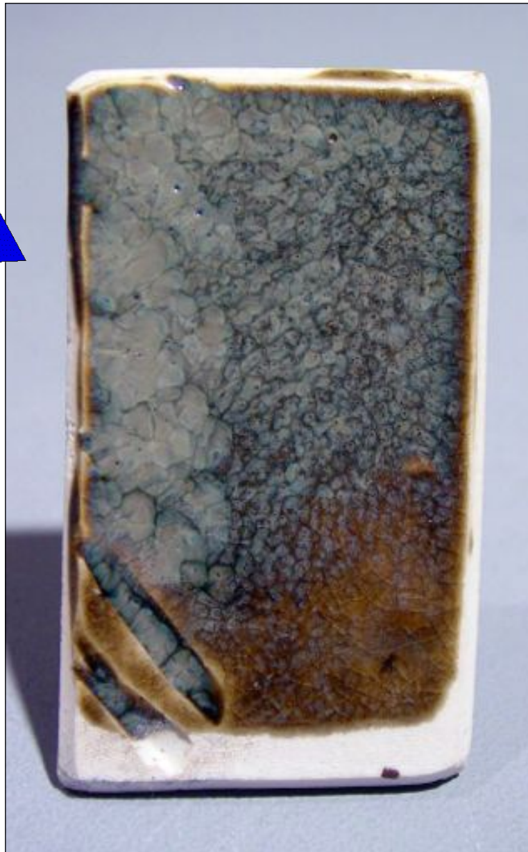
Falls Creek Ababi 6. The original recipe called for opacifier but it wasn't used in this test.
