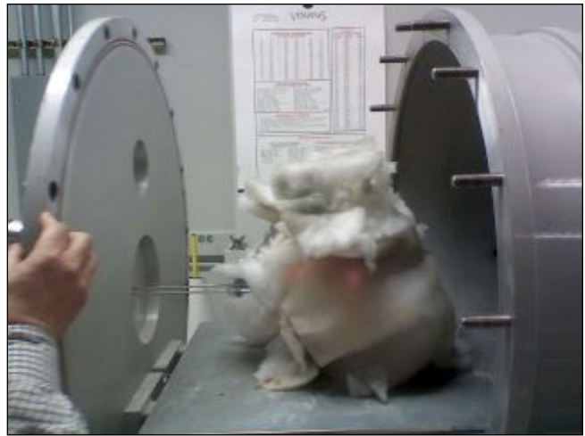
Fiber blanket was used to help retain heat and reach temperature faster.
