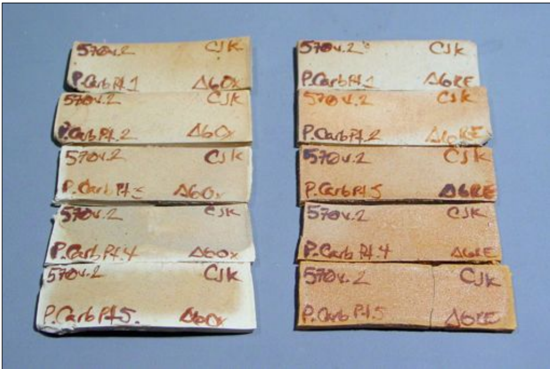
The #570 Variation 2 body with Pearl Ash additions in 2% increments from top to bottom. Oxidation on the left, reduction on the right.
