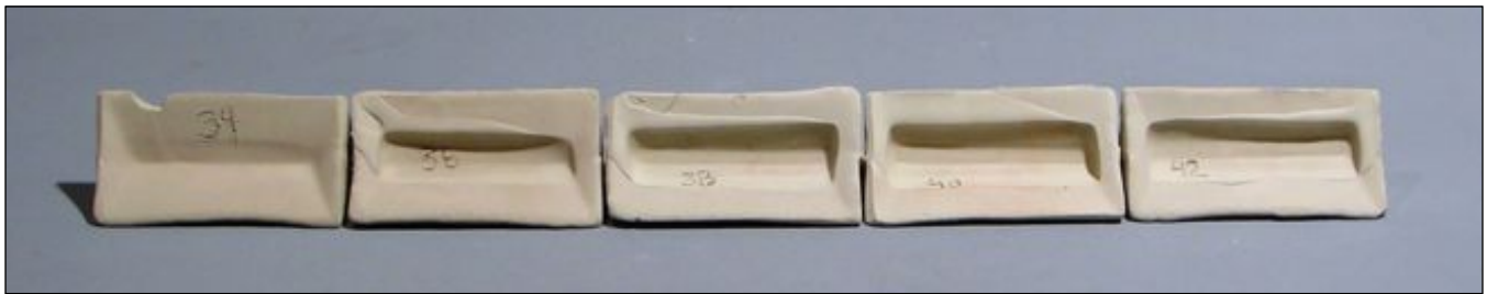
Castings done with increasing amounts of Darvan (drops of Darvan from left to right: 34, 36, 38, 40, 42).
