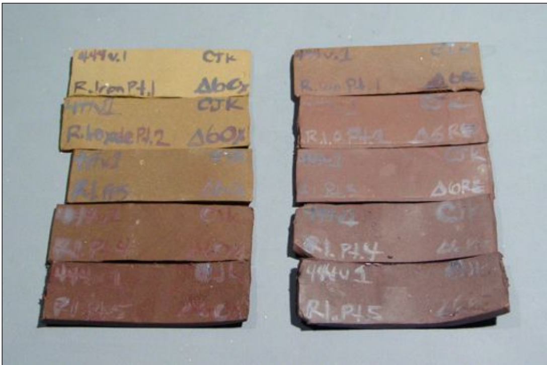
The #444 Variation 1 body with Red Iron Oxide additions in 2% increments from top to bottom. Oxidation on the left, reduction on the right.
