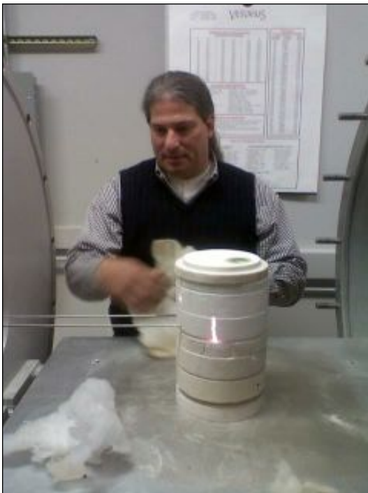
Crucible cooling after firing (note white-hot crack).
