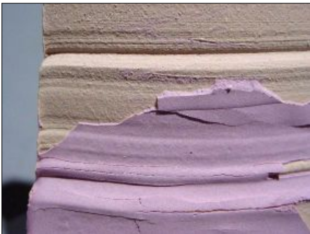
Detail of Mason Violet in New Zealand base. Flaking away sections reveal no contact with underlying clay surface.
