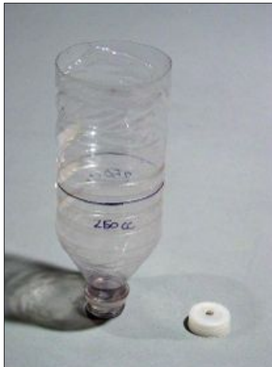
Homemade apparatus for recording the viscosity of slip.
