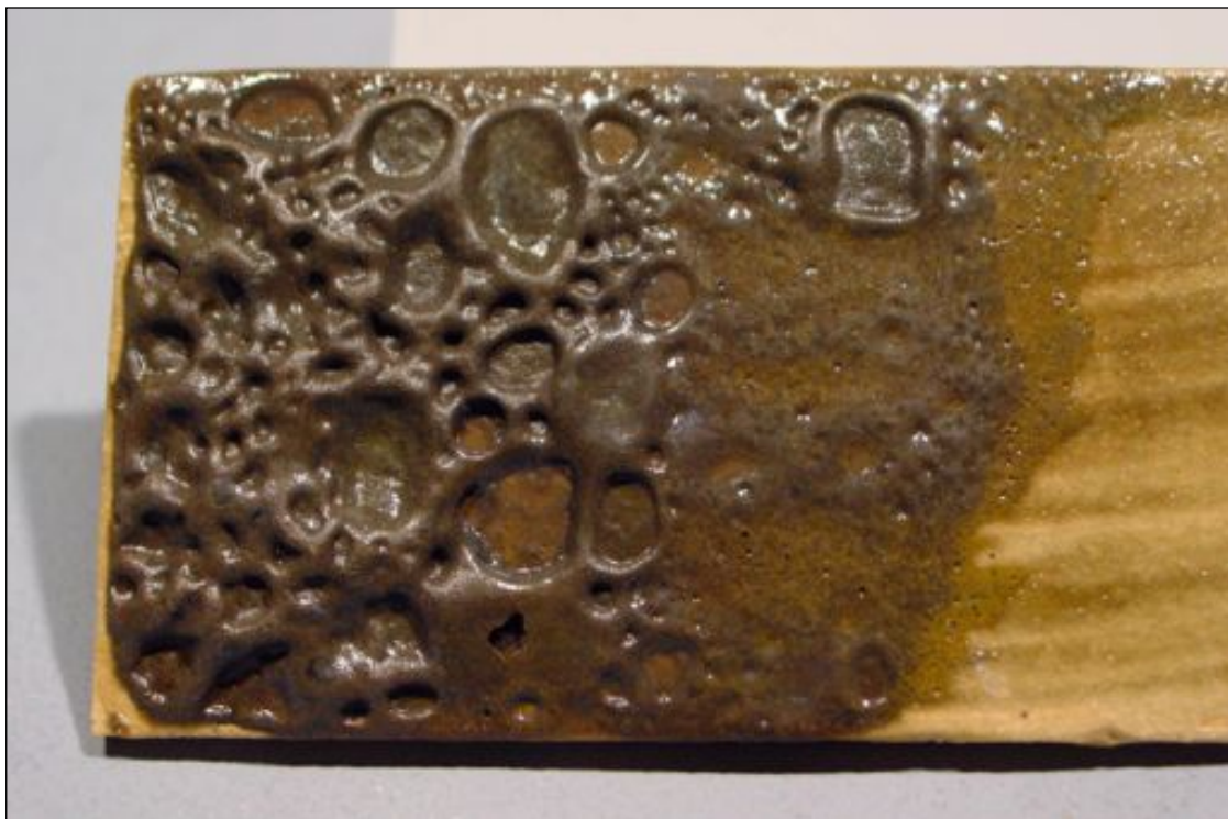
Detail of 5% addition of Copper Carbonate fired in oxidation. Under fired to cone 5. Note the small chip in the cratering toward the bottom due to handling. This only seems to happen at a medium thickness; the cratering is quite dense and strong where very thick and is nearly impossible to puncture with a fingernail.
