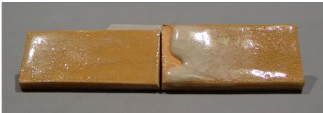
Comparison between adding 4% CMC (left) and Epsom Salt (right) in point 2. Note the difficulty in establishing thickness with the addition of 4% CMC.
