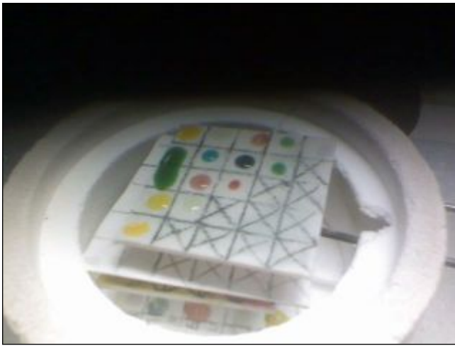
Pre fired tests loaded in sagger. Colors are due to food colorants added to each sulfate for easier visualization of the application process.
