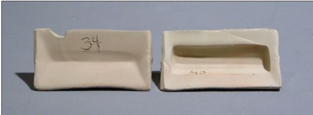
Castings done with 34 drops (0.86%) of Darvan on the left and 40 drops (1.016%) on the right. Note that the sample on the left coagulated, which prevented the slip from draining properly during casting. The additional Darvan on the right helped destroy this coagulation, allowing for better drainage.
