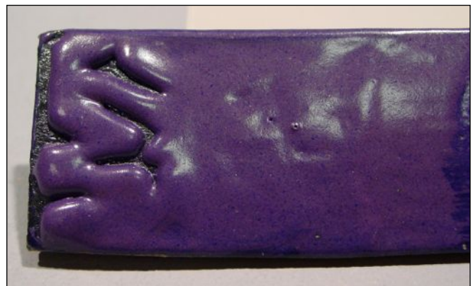
Details of 15% addition of Cobalt Carbonate in reduction and oxidation. Oxidation test was underfired to cone 5.
