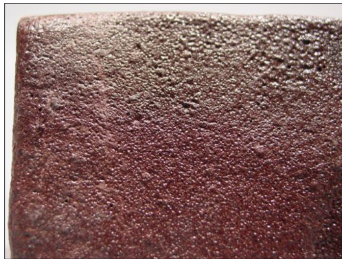
Detail of 5% addition of Crocus Martis fired in oxidation. Under fired to cone 5
