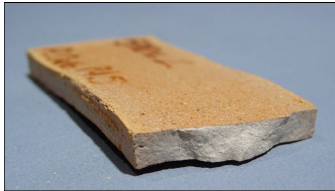
Cross-section of the above tile shows migration of Soda Ash to the surface.
