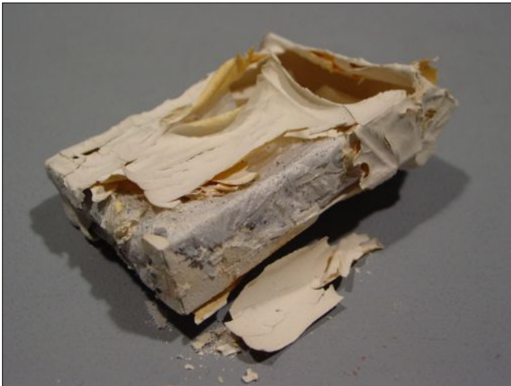
After addition on Epsom Salt. Note that the burning out of the paper destroys the slip.
