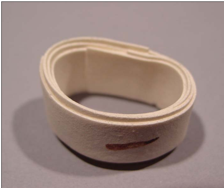
Close-up of single-thick tape laminated four layers thick
