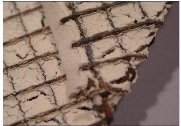
Fired examples of hardware cloth imbedded into tape during casting
