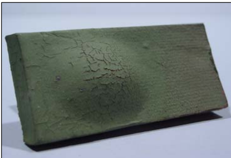
Large scale bloating (Chrome Oxide series)
