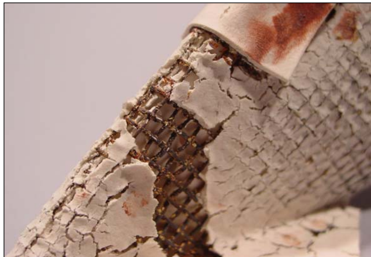
Fired example of window screen imbedded into tape during casting
