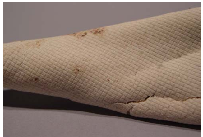
Fired example of window screen imbedded into tape during casting
