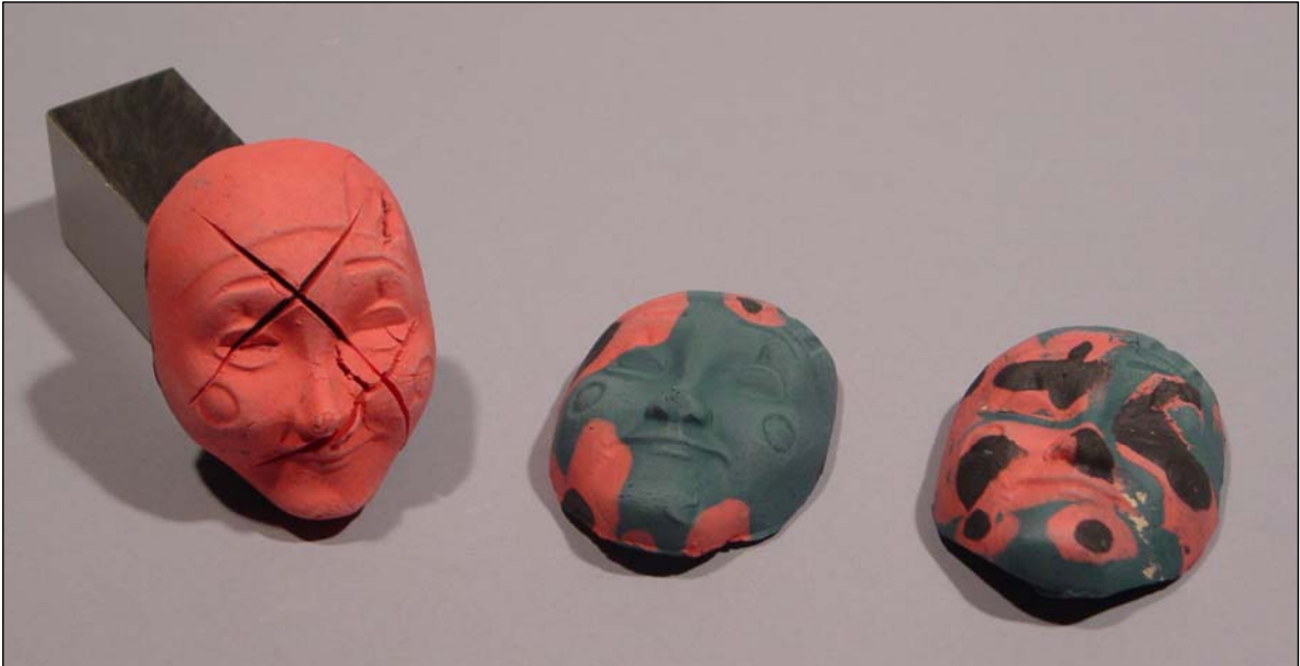
Colored bodies used in press molds
