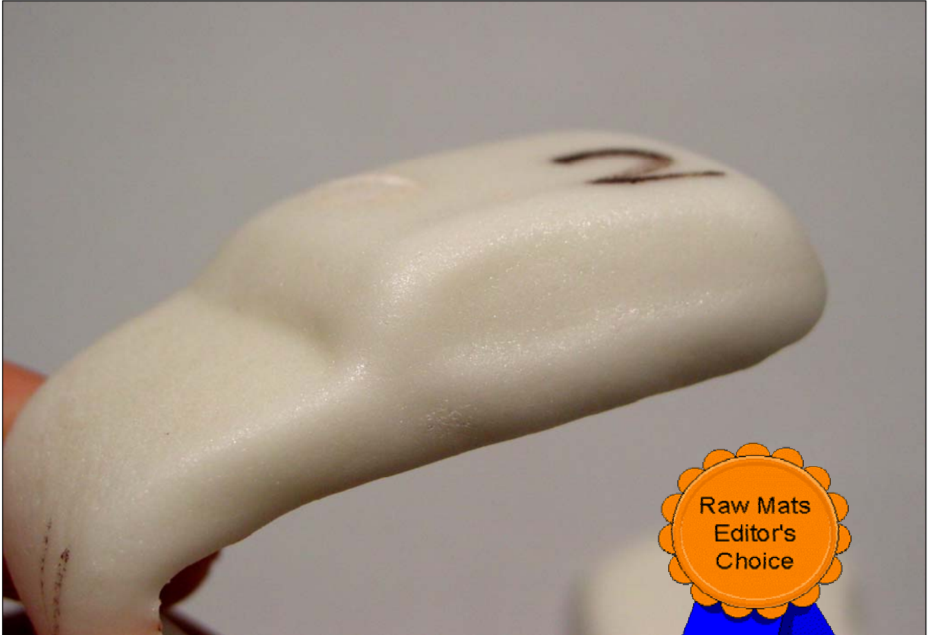
Point 2 From the Grolleg and frit 3110 blend (Test 3)
