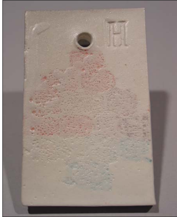
Various colors with clear glaze over top (poorly mixed and underfired)
