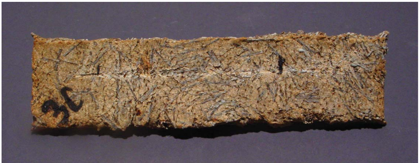
#444 body with 15% Fiberglass (3C)
