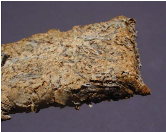
#444 body with 15% Fiberglass (3C)
