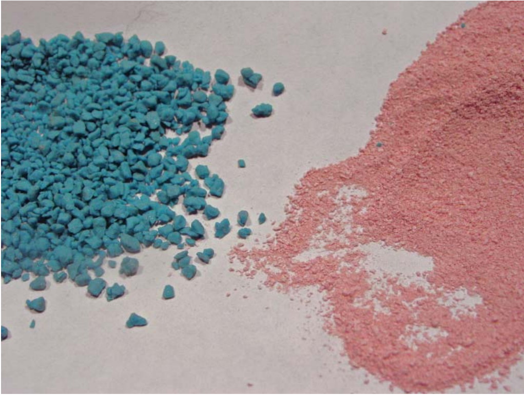
Fired blue and orange pitchers ready for addition to the base body
