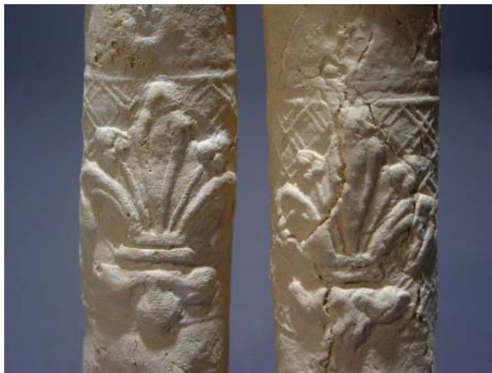
Fired results: Worked after re-hydrated... 5% wool (left) vs. 5% paper (right)
