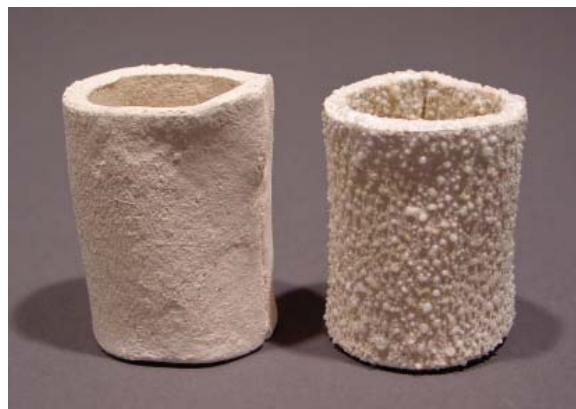
Point B at cone 05 (left) vs. point A at cone 3 (right)
