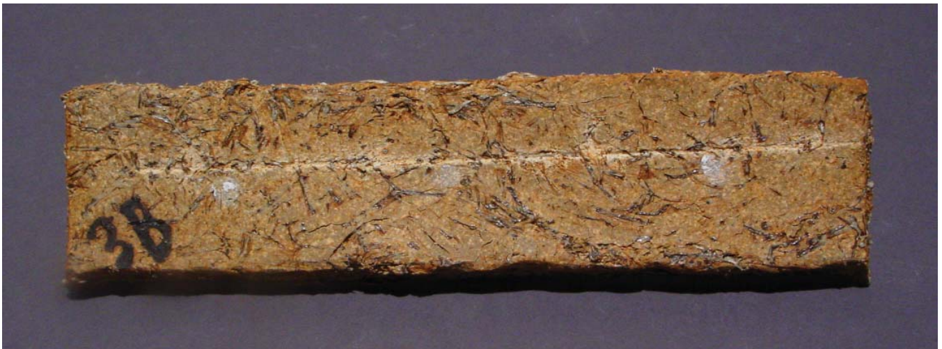
#444 body with 9% Fiberglass (3B)
