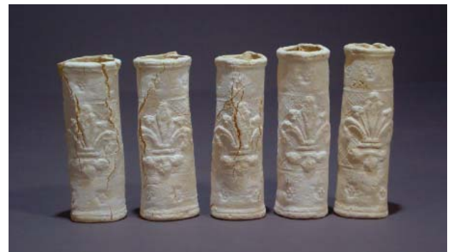
Fired results of wool rehydrated: additions of 0.25%, 0.5%, 1%, 2%, 5%
