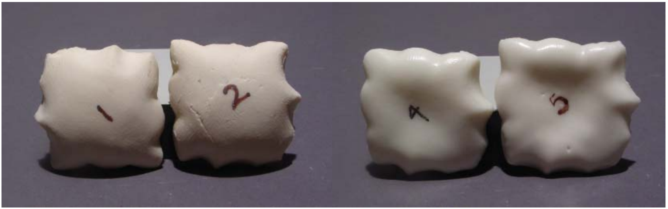
From first test (missing #3). Note the slumping with increasing amounts of flux.
