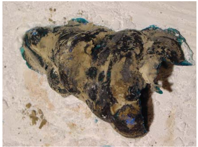
Chavarra #2 with 3% copper carbonate
