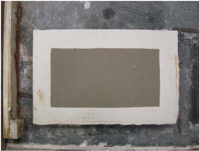
Creating a low-relief mold using a clay positive
