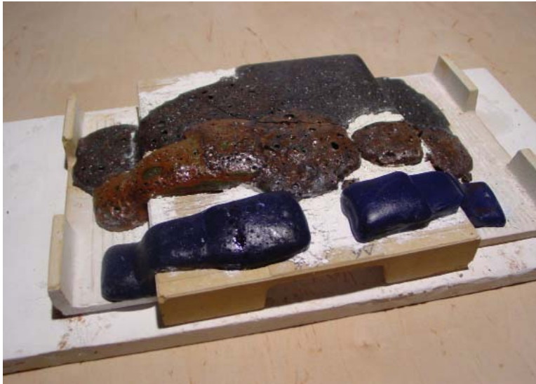
Copper and two of the cobalt results. Copper ran. Cobalt seemed more stable.
