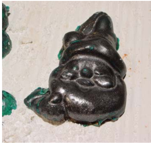
Chavarra #2 (modified) with 3% copper carbonate
