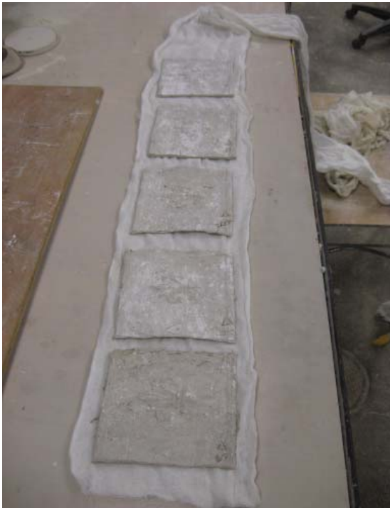
Drying the slabs by fully wrapping in cheesecloth
