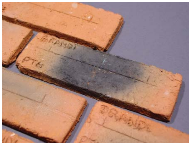
Discoloration in the samples is due to sawdust
