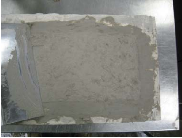
Mold troweled with flat scraper
