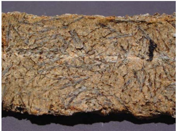
#444 body with 15% Fiberglass (3C)
