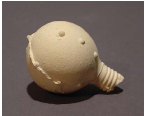
Vista Slip fired to cone 10
