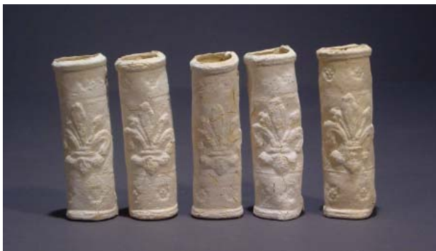
Fired results of wool worked wet: additions of 0.25%, 0.5%, 1%, 2%, 5%
