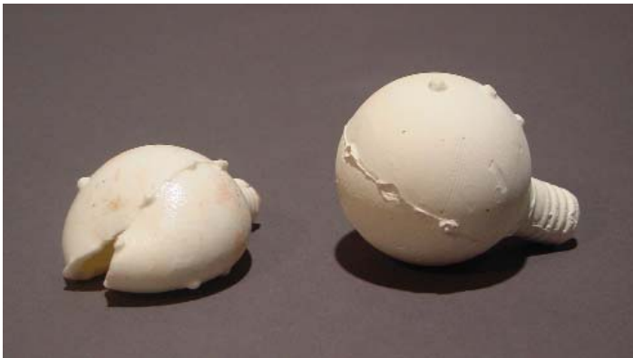
Porcelain Slip fired to cone 6 (left) and unfired (right)
