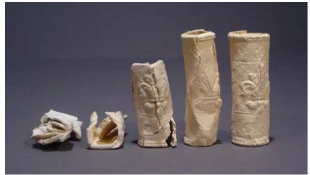
Fired results of paper re-hydrated: additions of 0.25%, 0.5%, 1%, 2%, 5%
