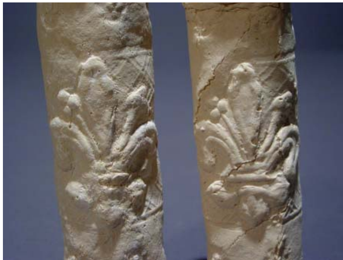
Fired results: Worked wet... 5% wool (left) vs. 5% paper (right)
