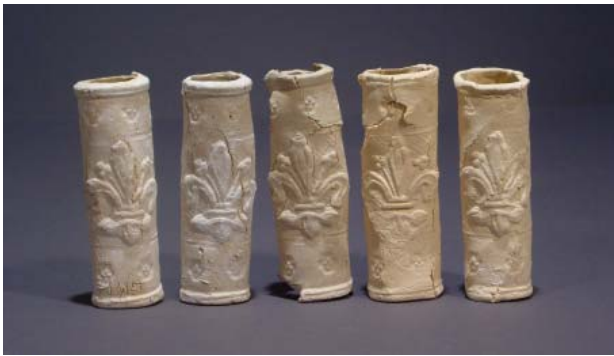
Fired results of paper worked wet: additions of 0.25%, 0.5%, 1%, 2%, 5%
