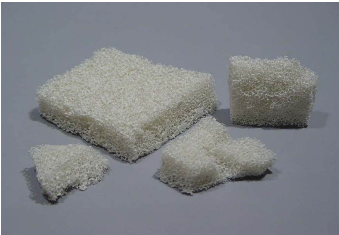
Reticulated plastic sponge dipped in thinner slip than above. Very thin network.
