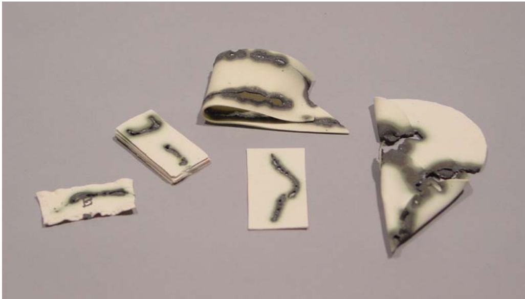
Fired porcelain tape with copper wire embedded right after casting
