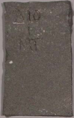
8% Black Iron Oxide 3% Manganese Dioxide 1% Cobalt Oxide
