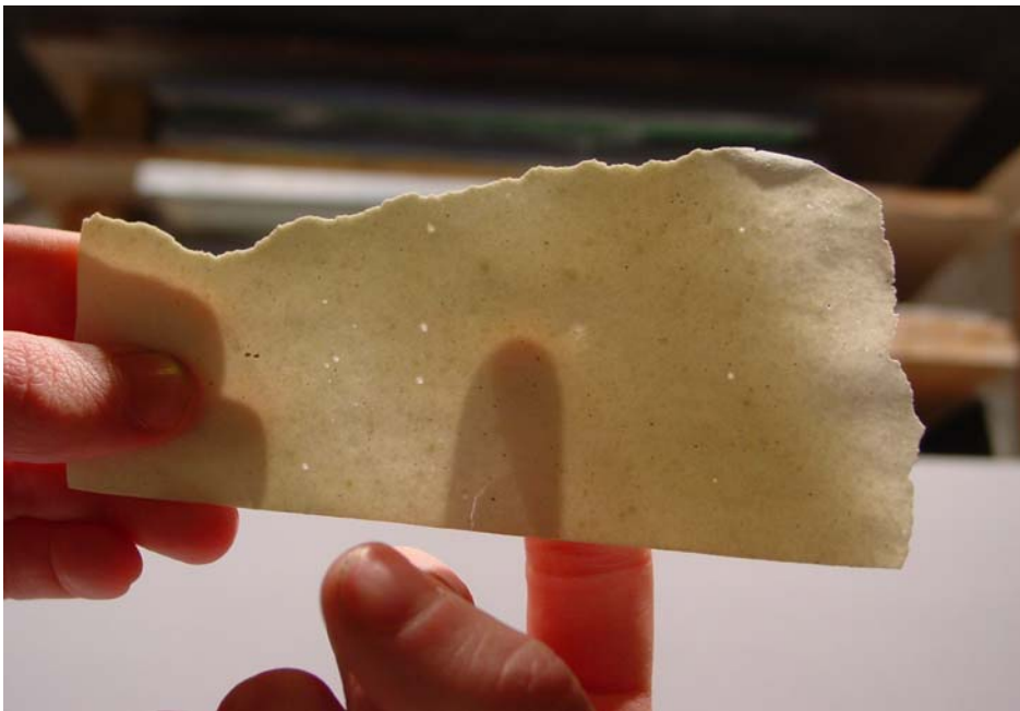
Despite being underfired, the tape is quite translucent
